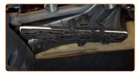
Install and secure the protective cover under the glove box.
