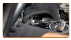
Install the engine cover and secure it. Make sure you hear a click indicating that it is locked in place.
