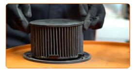
Install a new filter element into the holder, and then the entire assembly into the case, aligning the element upper part with the housing. Make sure that the filter edge fits tight to the housing.
