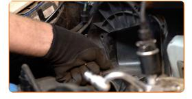
Screw the filter housing fastening bolts. Use HEX No.H5.
