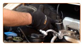
Remove the cabin air filter housing.
