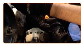
Release the air filter cover clips.
