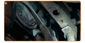
Replacement: serpentine belt – VW Transporter T4 Minibus (70B, 70C, 7DB, 7DK, 70J, 70K, 7DC, 7DJ). Tip:
