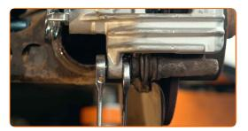
Remove the brake caliper. Use a crowbar.
