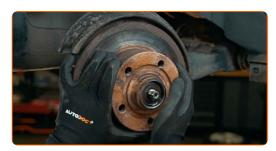
Clean the stub axle. Use a wire brush. Use all-purpose cleaning spray.
