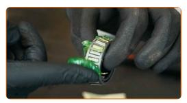
Press in the inner oil seal of the wheel bearing. Use a bush and bearing driver set. Use a hammer.
