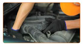
Screw the filter housing fastening bolts. Use a Phillips screwdriver.
