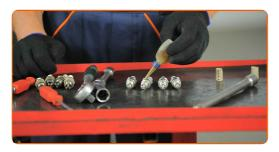
Install the new spark plugs into their mounting seats. Use the spark plug socket #21.
