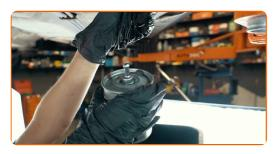
Remove the fuel filter bracket.
