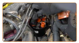
Replacement: distributor rotor – VW Transporter T3 Platform/Chassis. AUTODOC recommends:
