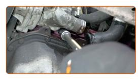
Remove the thermostat housing.
