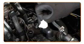
Attach the secondary air pump hoses.
