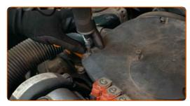
Remove the air filter housing.
