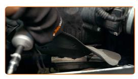
6 Detach the mass air flow sensor connector.
