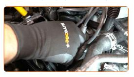
Replacement: ignition coil – VW Transporter IV Platform / Chassis (70E, 70L, 70M, 7DE, 7DL). AUTODOC experts recommend:
