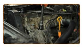
Replacement: spark plugs – VW Transporter IV Minibus (70B, 70C, 7DB, 7DK, 70J, 70K, 7DC, 7DJ). Professionals recommend:
