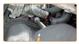
Remove the thermostat housing.
