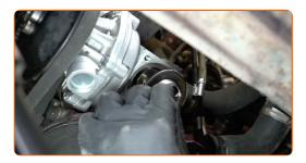
Replacement: engine thermostat – VW TRANSPORTER III Platform/Chassis. Tip:
