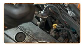
Replacement: spark plugs – VW TRANSPORTER III Platform/Chassis.
