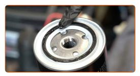
Screw the new filter into its place. Use a torque wrench. Tighten it to 23 Nm torque.
