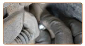
Remove the brake caliper. Use a crowbar.
