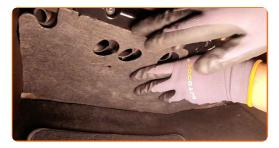
Screw in the fasteners of the bottom trim panel.
