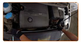
Detach the crankcase ventilation hose from the engine cover at the left.
