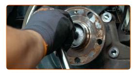
Remove the fastening bolt.
