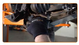
17 Remove the drive shaft from the wheel hub.
