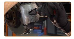
10 Remove the brake caliper.
