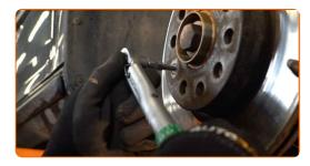
Install the brake caliper and fix it. Use HEX No.H7. Use a torque wrench. Tighten it to 30 Nm torque.
