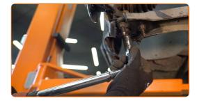
Install and tighten the drive shaft bolt. Use a drive socket #27.
