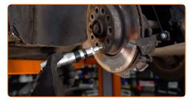
12 Remove the brake disc.
