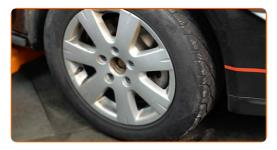
Tighten the bolt connecting the drive shaft to the wheel hub. Use a drive socket #24. Use a torque wrench. Tighten it to 200 Nm torque.+180°
