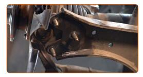
Tighten the ball joint fastener. Use a drive socket #16. Use a torque wrench. Tighten it to 60 Nm torque.
