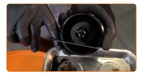
25 Screw the new filter into its place.
