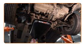
Clean the area of the oil pan drainage hole. Use a wire brush. Use WD-40 spray.
