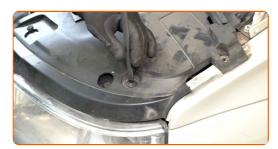
Unscrew the fasteners of the underbody cover panel. Use a drive socket #13. Use a ratchet wrench.
