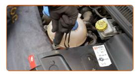
Attach the coolant expansion tank connector.
