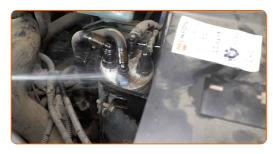
Disconnect the fuel supply lines from the fuel filter. Use a flat screwdriver.
