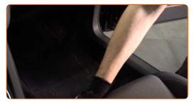
Unscrew the fasteners of the passenger side kick panel.
