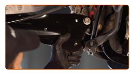
Tighten the fasteners connecting the control arm to the rear knuckle. Use a drive socket #18. Use a torque wrench. Tighten it to 90 Nm torque.+90°
