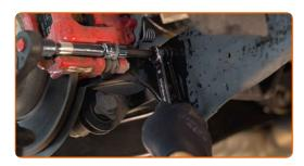
Remove the retaining clip of the parking brake cable. Use a pin punch. Use a hammer.
