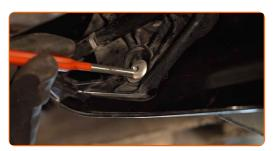
Install the rod fastening to the stabilizer and tighten it. Use a combination spanner #16. Use a drive socket #16. Use XZN #6. Use a torque wrench. Tighten it to 45 Nm torque.
