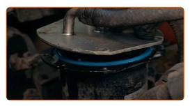
Remove the fuel filter. Use a flat screwdriver.
