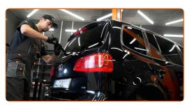
Press the clip. Remove the blade from the wiper arm.
