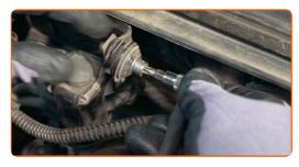
6 Unscrew the brake fluid reservoir cap.
