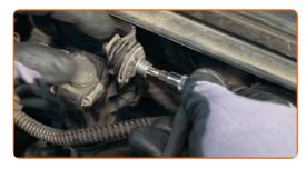
6 Unscrew the brake fluid reservoir cap.
