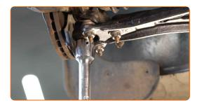
Tighten the front fastener connecting the control arm to the subframe. Use a drive socket #18. Use a torque wrench. Tighten it to 70 Nm torque.+180°
