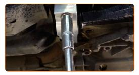
Screw the rear fastener connecting the control arm to the subframe. Use a drive socket #16. Use a ratchet wrench.
