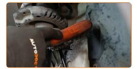
Unscrew the fastener connecting the stabilizer link to the shock strut. Use a drive socket #19. Use a ratchet wrench.
