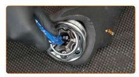
Move the inner race of the new CV joint from side to side to get it ready to work.
