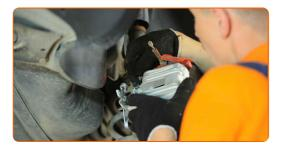
Secure the parking brake cable with the retaining clip. Use a flat screwdriver.
