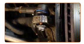
Screw on the tie rod end jam nut. Use a combination spanner #22. Use a combination spanner #24.
