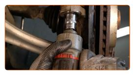
Disconnect the tie rod end from the steering knuckle. Use a ball joint puller.
