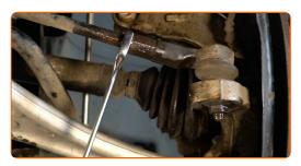
Unscrew the end fastening nut to the steering knuckle. Use a drive socket #18. Use a tap wrench.
