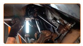
Tighten the fastener connecting the stabilizer link to the stabilizer bar. Use HEX No.H5. Use a combination spanner #17. Use a torque wrench. Tighten it to 40 Nm torque.
