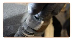
Tighten the brake caliper fasteners. Use a drive socket #13. Use a torque wrench. Tighten it to 35 Nm torque.
