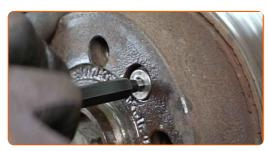
Remove the fastening bolt.
