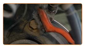
Unscrew the caliper bracket fastening. Use a drive socket #18. Use a ratchet wrench.
