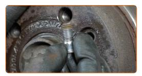
Remove the brake disc.
