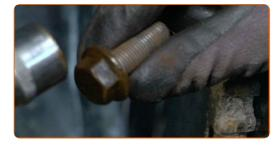
Remove the caliper bracket.
