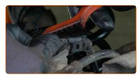
Detach the connector of the brake pad wear sensor.
