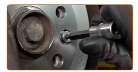
Tighten the brake disc fastening. Use HEX No.H6. Use a torque wrench. Tighten it to 10 nm torque.
