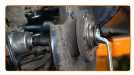
Remove the fastening bolt.
