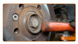
Unscrew the brake disc fastening. Use HEX No.H6. Use a ratchet wrench.
