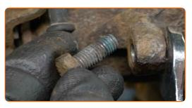
Remove the brake caliper. Use a crowbar.
