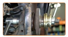
Install the spring washer with a reluctor ring.
