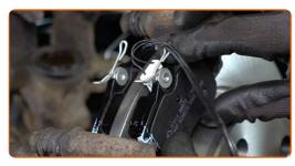
Install the brake caliper and fix it.
