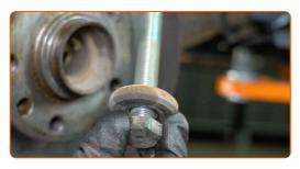
Remove the spring washer with a reluctor ring.
