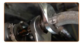
Unscrew the end fastening nut to the steering knuckle. Use a drive socket #18. Use a ratchet wrench.
