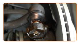
Set the tie rod end to the correct position and secure it with the lock nut. Use a vernier caliper. Use a combination spanner #22 (2 pieces).
