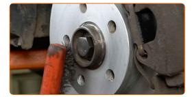
Treat the surface where the brake disc contacts the wheel rim. Use ceramic grease.
