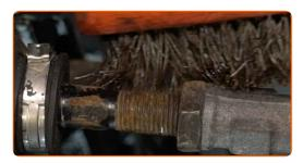
Loosen the lock nut securing the tie rod end to the tie rod. Use a combination spanner #22 (2 pieces).
