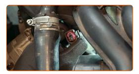
Unscrew the alternator power cable fastener. Use a combination spanner #13.
