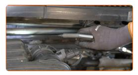
10 Install a new filter element into the frame.
