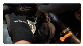
Remove the o-rings. Use a flat screwdriver.
