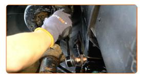
Screw in the sway bar link fasteners. Use a combination spanner #16. Use a drive socket #19. Use a ratchet wrench.
