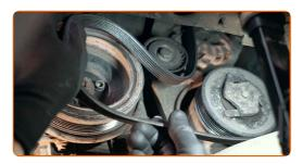
Return the tensioner pulley to its initial position. Use a combination spanner #16. 10
