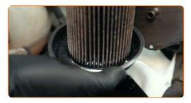
Pump the fuel out of the fuel filter housing. Use a hand-operated fluid syringe.
