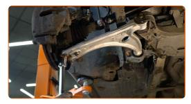
Tighten the front fastener connecting the control arm to the subframe. Use a drive socket #18. Use a torque wrench. Tighten it to 70 Nm torque.+180°
