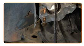
Screw the rear fastener connecting the control arm to the car body. Use a drive socket #18. Use a ratchet wrench.
