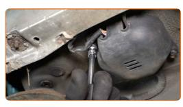
Remove the oxygen sensor housing cover.
