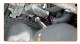
Remove the thermostat housing.
