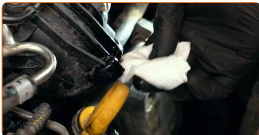
**55** Install the throttle valve on the intake manifold. Install the fastening bolts.
