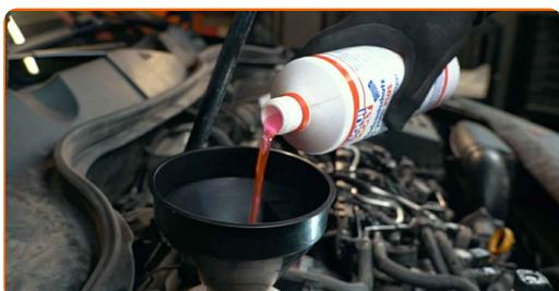
Replacement: engine thermostat – VW Scirocco III (137, 138). Tip from
