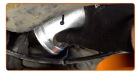
Attach the fuel filter fasteners. Use nippers.
